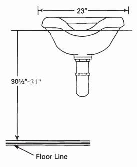
The depicted mounting height is the recommended mounting height for bowls of this design when used hydraulic all-purpose chair.
