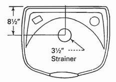
Fasten mounting plate to wall. Place bowl on top of plate flange with back side of bowl against leveling bolt. Use two 5/16" - 18 x 1/2" rd. hd. screws with 3/8" x 1" washers to fasten plate flange to underside of shampoo bowl. (Do not overtighten.)
